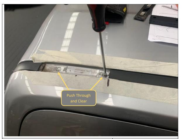
13. Using a small screwdriver or pick, push through the factory sealant patches covering the threaded mounting points in the roof.
