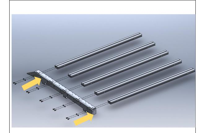
16. Fit the side rail to the extrusion,
