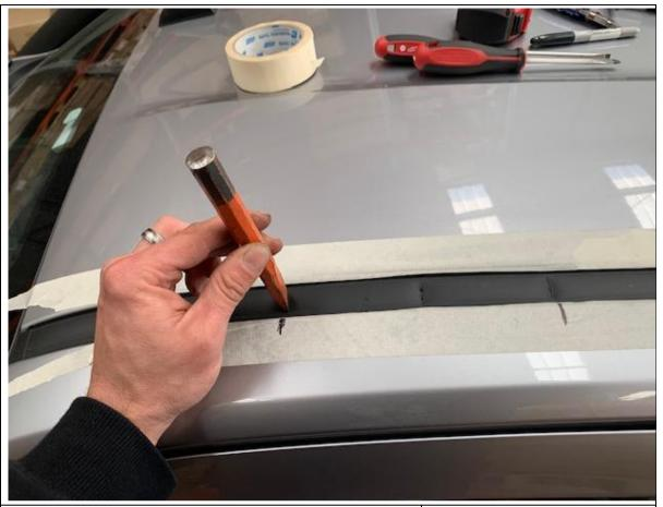
Using a cold chisel, carefully strike the roof rubbers at the front and rear points measured earlier. These initial strikes should be reasonably gentle such that they cut the rubber and score the metal strip embedded within.
